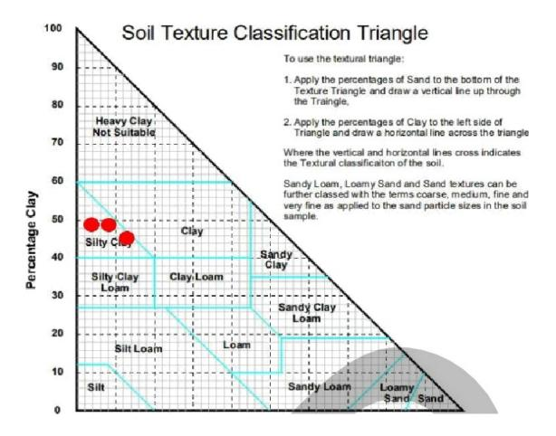
Based on the Soil Texture Classification Triangle provided in Alberta Private Sewage Standard of Practice, the tested soil is classified as Silty Clay.
