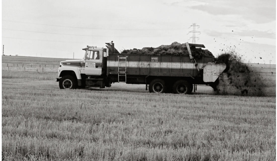
Figure 19. A custom spreader being used to spread large amounts of manure.
