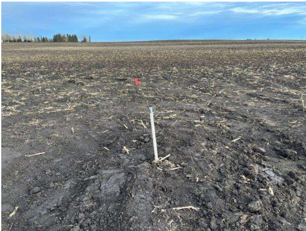
12. View of the geotechnical stand pipe piezometer located in the northcentral portion of the Project Site; photograph taken facing east.
