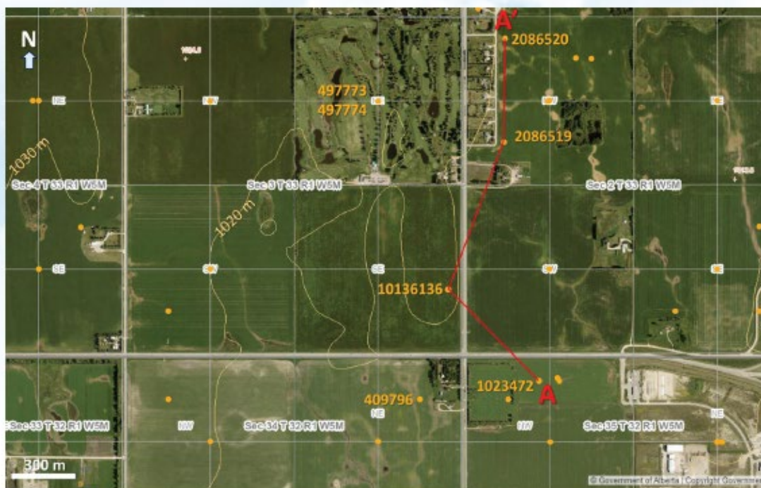
FIGURE 3 Aerial photo with surface topography contours and A-A' cross section well locations
