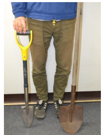
Figure 4. Tree planting shovel (left) and generic spade (right). Photo by AWES.
